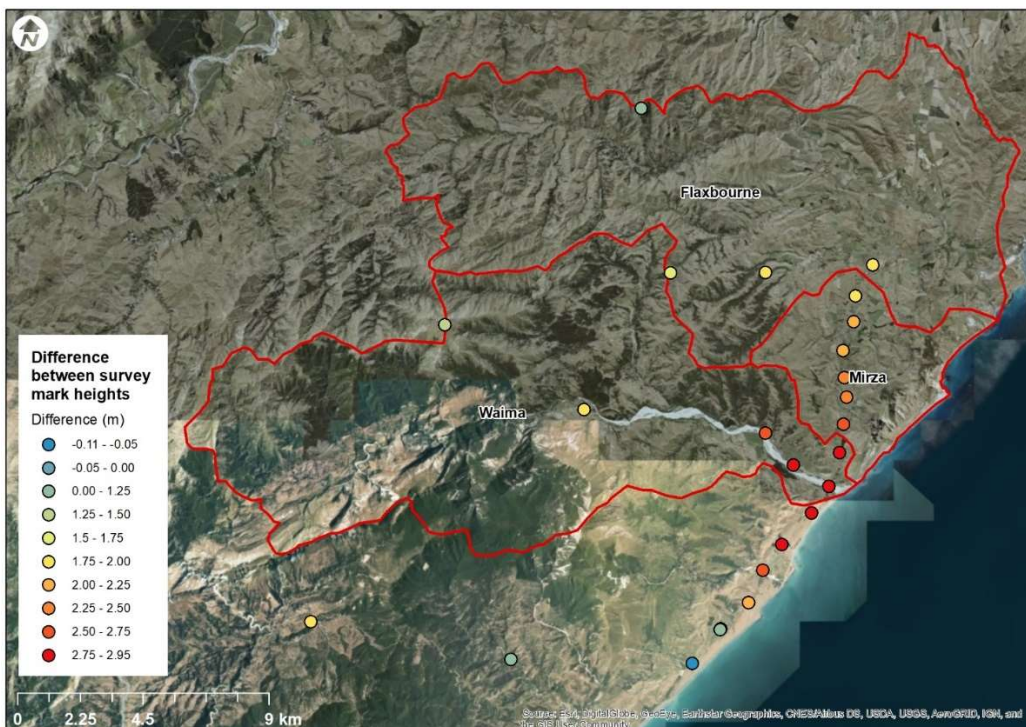
Figure 4.4: Comparison of the elevations of pre-earthquake geodetic benchmarks and post-earthquake LiDAR.
